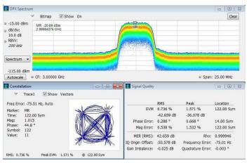
Multi-domain views provide a new level of insight into design or operational problems not possible with conventional analysis solutions. Here vector modulation quality and constellation (Opt. 21) are combined with the continuous monitoring of the DPX® spectrum display.
