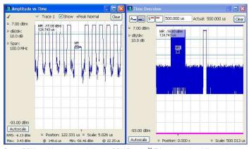
Swept DPX combines the revolutionary DPX Density™ Trigger with the ability to trigger on runt pulses and apply time qualification to any trigger. The runt trigger seen here can be used to track down nonconforming pulses in a pulse train, greatly reducing time to insight. Time qualification can be used to separate ranging pulses from higher resolution pulses in a radar signal, or trigger only on signals that remain on longer than a specified time.
